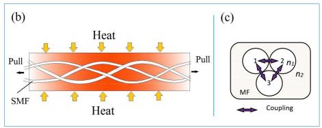
**Figure 1.** (a) Schematic diagram of the proposed sensor; (b) Three fibers are slightly twisted together to ensure close proximity among them during the fusing and tapering process. (c) Sketch of a cross-section of the  $3 \times 3$  tapered microfiber coupler (Tri-MFC) immersed in magnetic fluid.
