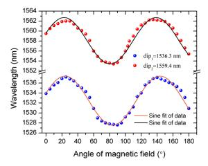
**Figure 5.** Periodic change in the position of spectral dips with initial positions at 1536.3 nm and 1559 nm when the applied magnetic field direction changes from 0 two 180 degrees.
