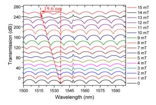
**Figure 3.** Experimental output spectra for the sensing head immersed in a MF containing 12 nm-diameter Fe<sub>4</sub>O<sub>3</sub> particles with concentration of 5 mg/mol at different magnetic field strengths ranging from 0 to 15 mT.
