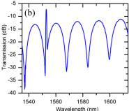
**Figure 2.** (a) Interference spectrum of polarization maintaining fiber - microfiber coupler (PMF-MFC) loop measured at port 2 without the fiber Bragg grating (FBG); (b) Combined spectra of the FBG and the PMF-MFC loop measured at port 2.
