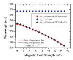
**Figure 4.** Measured wavelength shift of the selected transmission dip (at 1536.3 nm) and the FBG reflection peak (1547.6 nm) against increasing magnetic field from 0 to 15 mT and then decreased back to zero.
