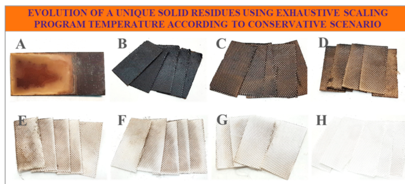
Figure 4. Thermal degradation over time of resin within a unique solid residue from the HTD process, using a scaling program with the highest temperature going from 355 to 550 °C according to the conservative scenario (A,B,C,D,E,F,G, and H for original solid residue R_30, 480 min at 355 °C, 60 min at 375 °C, 30 min at 400 °C, 20 min at 425 °C, 12 min at 450 °C, 1 min at 500 °C, and 1 min at 550 °C, respectively).
