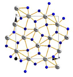
From the experimental findings of Zerr *et. al.*, the orthorhombic  $Ta_2N_3$  displays high hardness and a unique texture and this makes it a potential superhard material for industrial applications.
