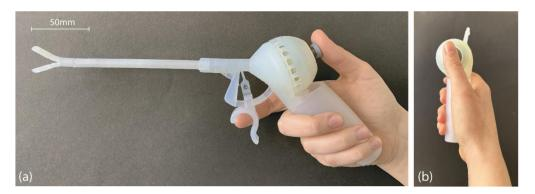
**Figure 7.** The assembled prototype. (a) Front view, (b) side view that shows the alignment of the wrist and the thumb.
