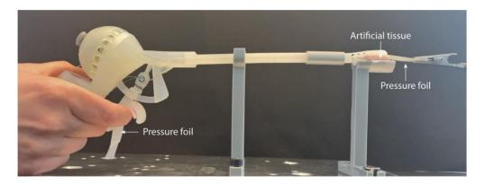
**Figure 11.** Set-up of the grasping force measurement.
