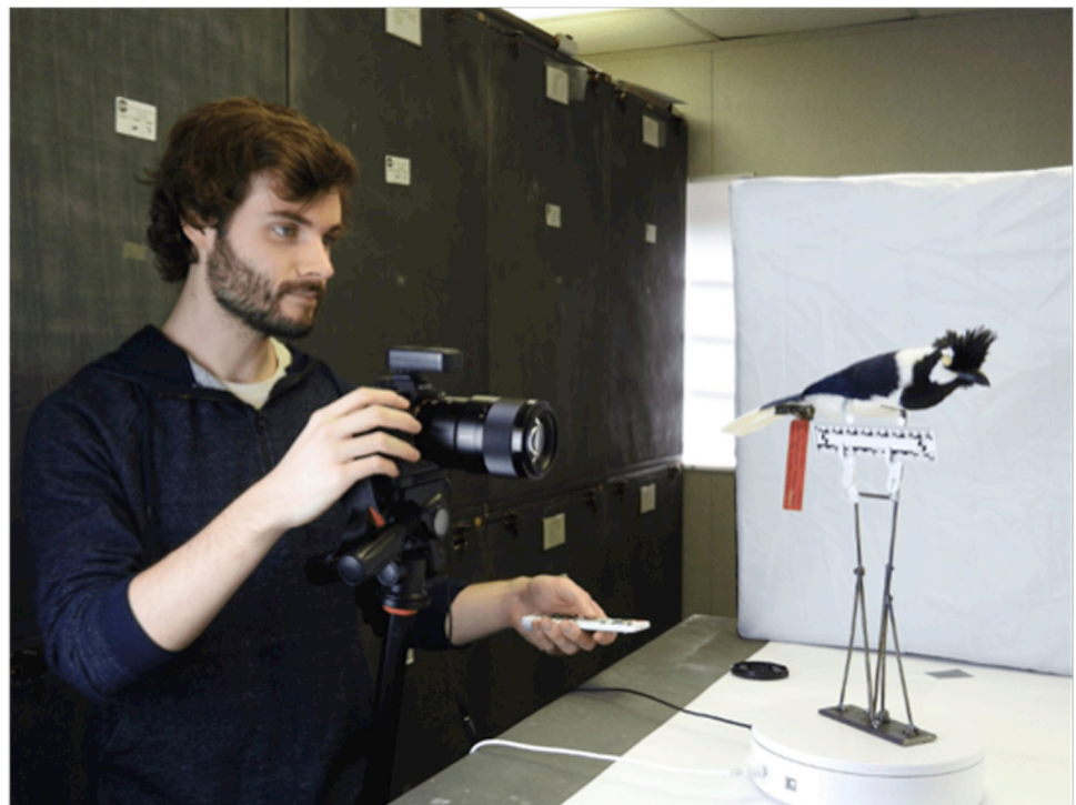
Fig 1. One of the authors with the physical set-up, showing the stand on top of a turntable with shutter integration to a camera on tripod. The ruler sits just below the specimen. Softbox light sources (one shown) are placed on both sides of the specimen. The specimen shown is the holotype of the Tufted Jay ( Cyanocorax dickeyi ), MLZ:Bird:12342.
