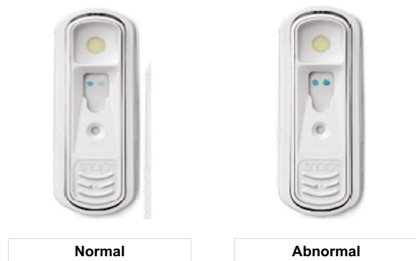
Fig 1. Image of the N-terminal prohormone of brain natriuretic peptide Point-of-Care SNAP ELISA showing normal and abnormal results. Image is courtesy of IDEXX Laboratories, Inc. b
