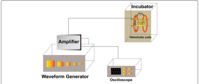
**Fig. 1** Schematic diagram of EMF device. The facility consists of four main parts: waveform generator, amplifier, two Helmholtz coils, and oscilloscope. EMF frequency verified by oscilloscope as consistent and sinusoidal. Helmholtz coils which produced uniform EMF placed in an incubator (37 °C, 5% CO<sub>2</sub>), and cell culture plates placed in center of coils
