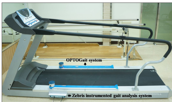
Figure 1. Lateral view of the 2 measuring systems. The transmitting bar and receiving bar of the OPTOGait system were placed on the side bars of the Zebris treadmill.
