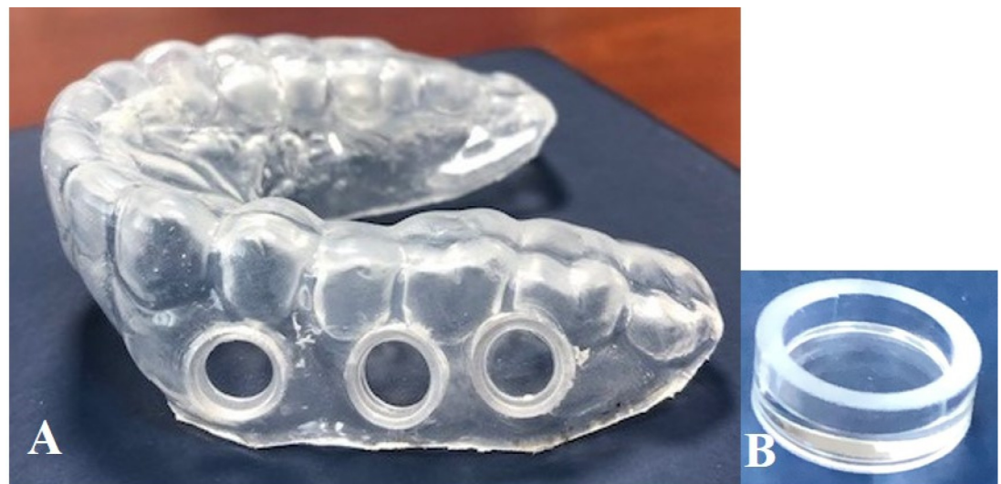
Fig 1. The intraoral device for in-situ biofilm collection. A: Intraoral device with removable wells, showing three different pits where the removable wells are inserted; B: An image of a removable well submerged within the dimensionally fitting well in the device.
