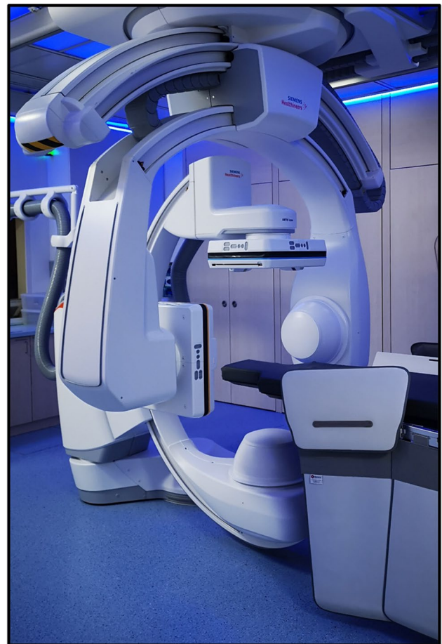
Fig. 2 HS-FD-CT scanner: biplane angiography system with mounted FD-CT
