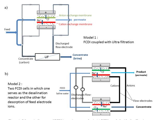
**Figure 9.** Schematic diagrams of FCDI in continuous mode via (a) FCDI coupled with ultrafiltration and (b) two FCDI cells.
