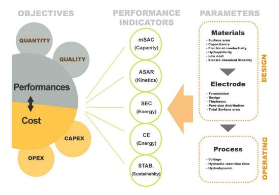
Figure 6. Schematic diagram of CDI performance indices.
