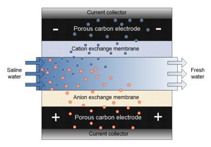
Figure 7. Schematic representation of membrane capacitive deionization (MCDI) system.
