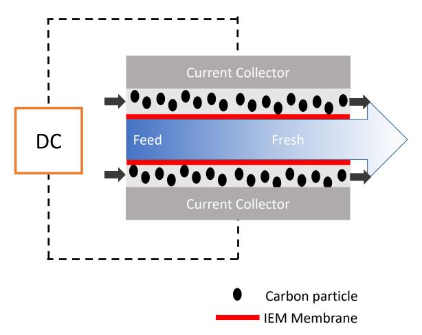
Figure 8. Schematic representation flow capacitive deionization (FCDI) system.
