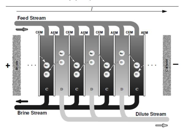
**Figure 2.** A schematic diagram of electrodialysis (ED) where C is the concentrate compartment and D is the dilute compartment.
