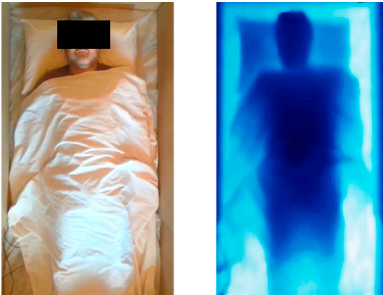
Figure 1. An RGB image of a subject under a sheet ( left ) and its corresponding depth image ( right ).
