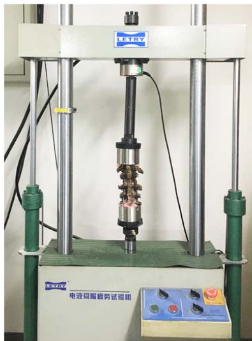
Figure 3. Cyclic load test. Cyclic compressive loading was performed vertically aligned along the vertebral axis. The fatigue testing machine was set to a cyclic loading state with the following loading schedule: 3 h total, cycle of 60/min, 10,000 revolutions, initial pressure of 300 N, peak pressure of 3,000 N, front flexion of 8^\circ .
