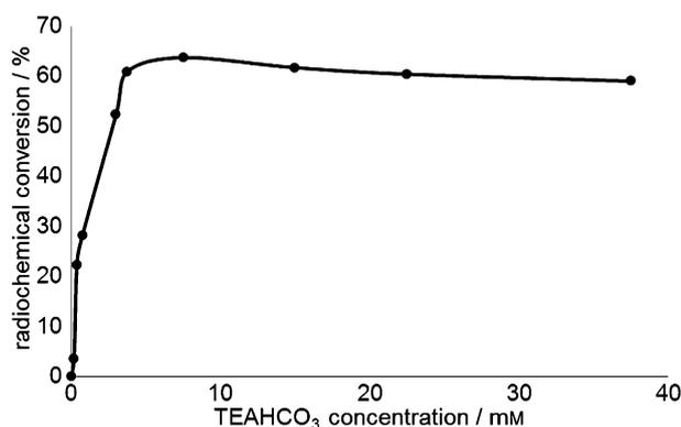
**Figure 2.** Correlation between TEAHCO<sub>3</sub> concentration and radiochemical yields in the ring opening of Boc-activated methylaziridine-2-carboxylate with [<sup>18</sup>F]fluoride (reaction conditions: 5 mg precursor, DMSO, 130 °C MW, 10 min).
