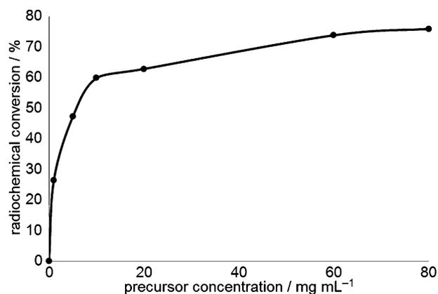
Figure 1. Correlation between Boc-activated methylaziridine-2-carboxylate concentration and radiochemical yield in ring opening with [<sup>18</sup>F]fluoride (reaction conditions: TEAHCO<sub>3</sub>, DMSO, 130 °C MW, 10 min).
