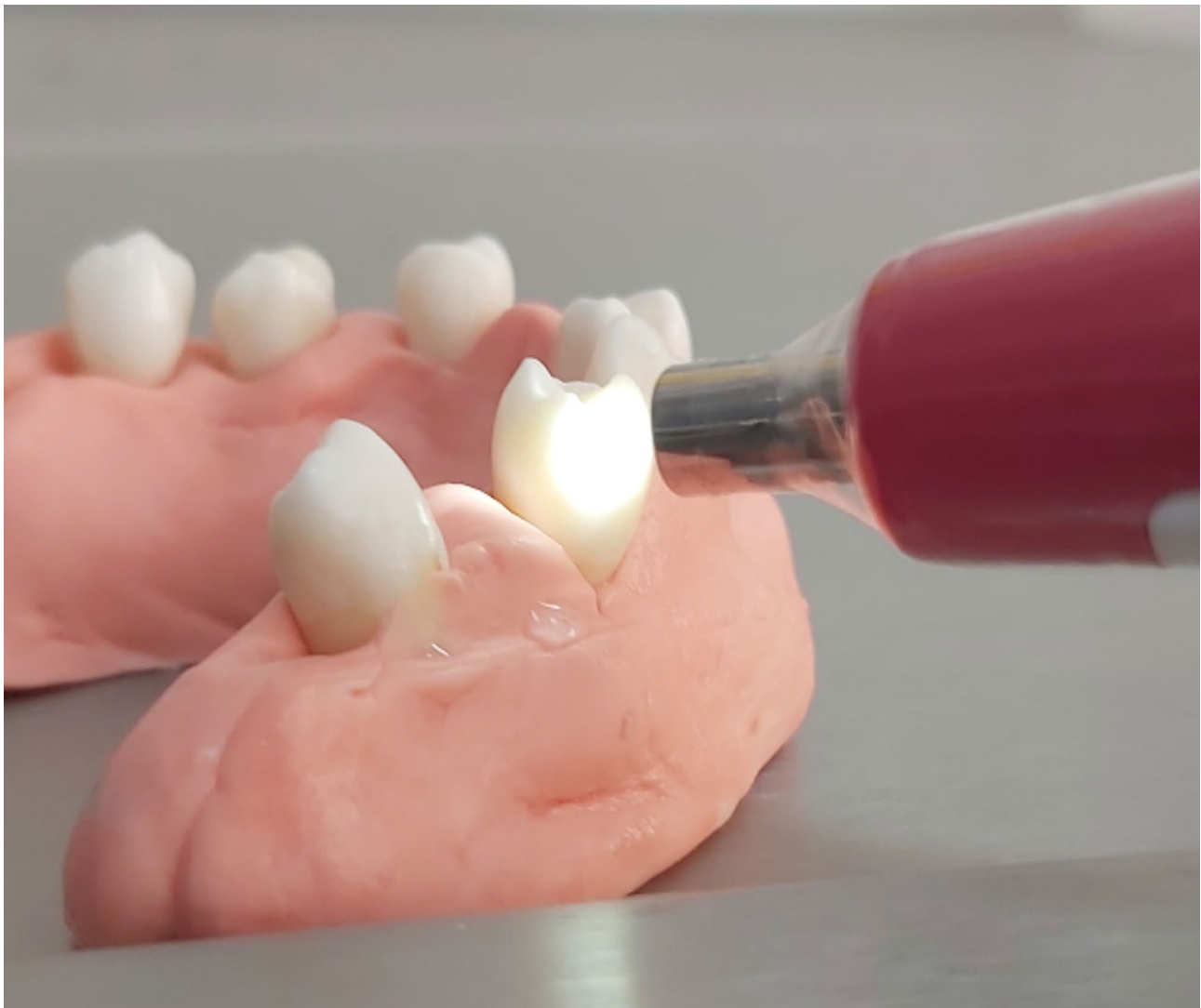
Fig. 2 \Delta E value was measured using spectrophotometer
