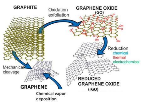
Figure 1. Schematic representation of graphene-related materials (GRMs) and their synthesis methods.
