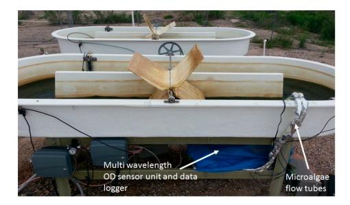
**Figure 3.** Optical sensor integrated into an open pond raceway for real-time microalgae growth monitoring.
