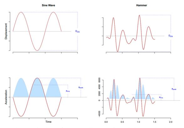
**Figure 2.** Displacement and accelerations for sine wave and hammer oscillations: displacement and accelerations are only mathematically related for sinusoidal oscillations. Abbreviations: p2p = peak-to-peak; RMS = root-mean-square.
