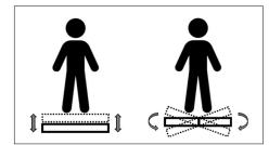
Figure 1. Standing on a platform with vertical vibrations (left) versus side-alternating vibrations (right).
