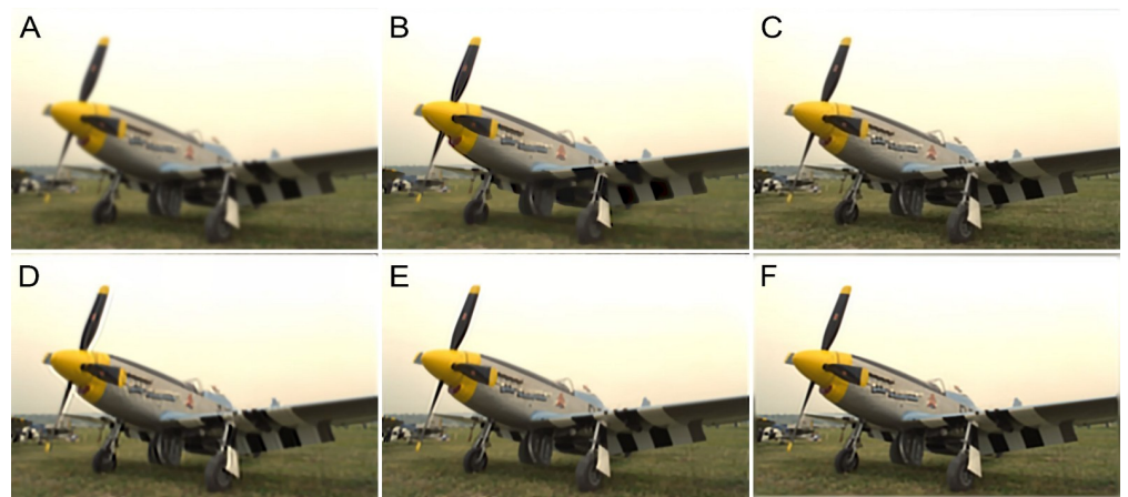
Fig 16. Atmospheric turbulence blur with \sigma = 3.2 for the “plane.bmp” image. (A) Blurred image. (B) Method in [49]. (C) Method in [50]. (D) Method in [51]. (E) Method in [52]. (F) Proposed method.
