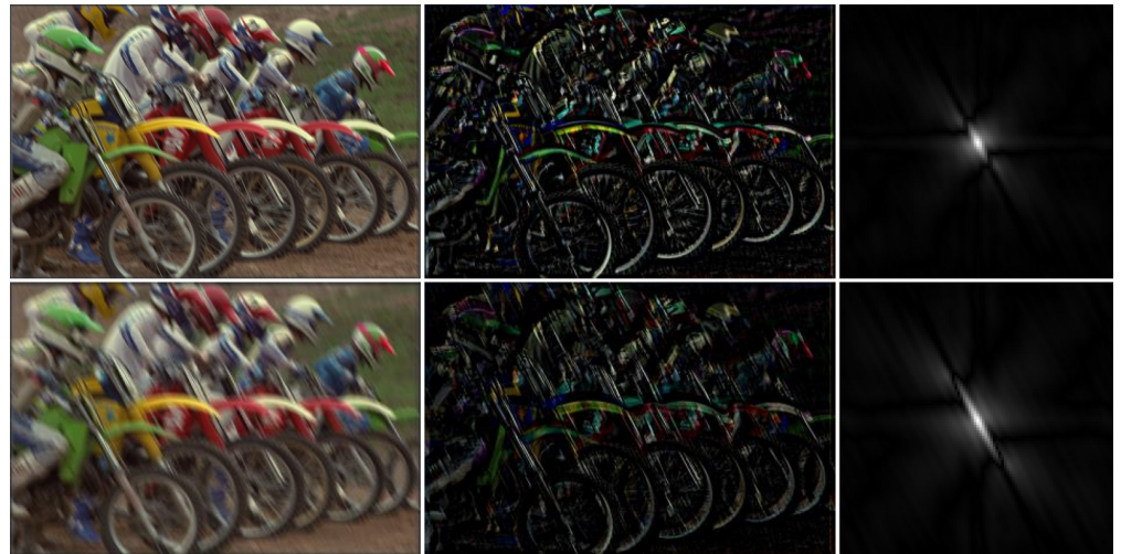
Fig 3. Examples of the blur feature in motion blur. Left: Motion blur of the “bikes.bmp” image with L = 10 (first row) and L = 20 (second row) and orientation \Phi = 120^\circ . Middle: Gradient domain. Right: Amplitudes of the blur features.
