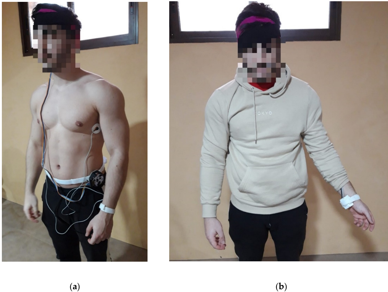
Figure 7. (a) Placement of each of the elements that make up the ambulatory monitoring system on the user; (b) Final arrangement of the ambulatory monitoring system on the user with clothing. It can be seen that the design is unobtrusive and produces practically no disturbance to the user's daily activities.
