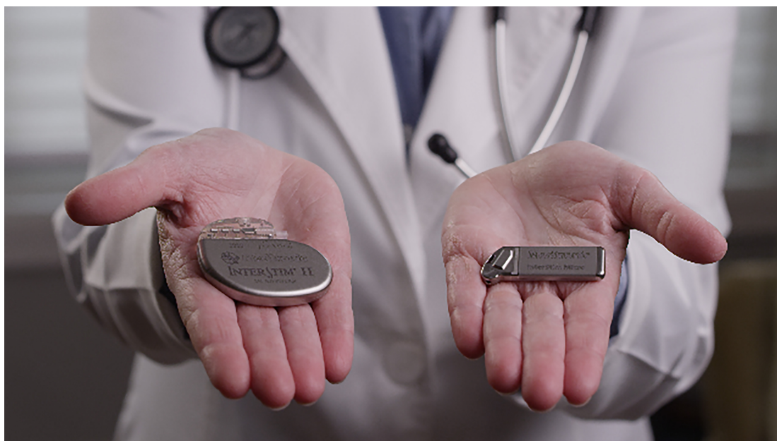
Figure 1 - Size difference between the InterStim™ II (non-rechargeable) and the InterStim™ Micro (rechargeable) implantable pulse generators.
