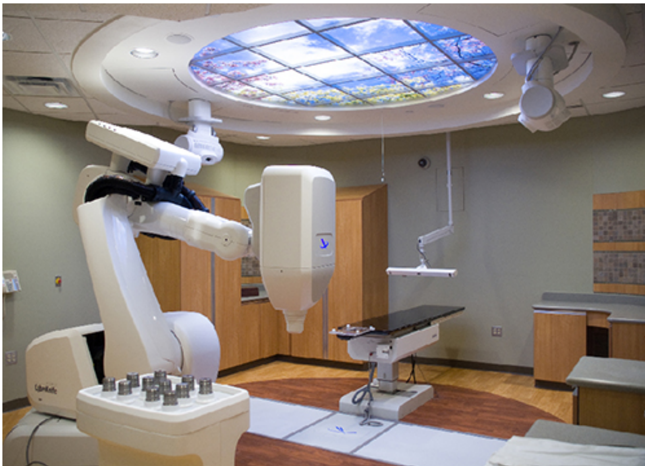
Figure 1. Cyberknife system. A view of the Cyberknife system used for the measurements, with the accelerator head pointing downwards. The water tank can either be placed on the floor, or on the robotic couch visible at the back of the room, depending on the space available above the head.
