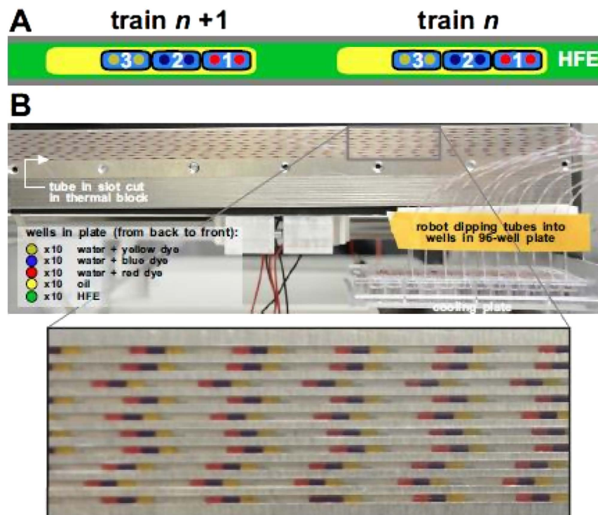
Figure 6. High-throughput generation of hundreds of DIBs. Ten 480- \mu\text{m} tubes are attached to 10 syringes driven by one pump; the other ends of the 10 tubes are dipped by a robot successively into appropriate fluids in a 96-well plate to generate a series of identical trains (each with three 200-nl water drops containing a dye of different colour). Flow packs drops coated with monolayers against each other to create 2 DIBs/train. (A) Fluidic architecture of two of the identical trains in series in one tube (fluids –HFE7500, water + red, blue or yellow dye, and tetradecane +3% EM180). (B) A still from Movie S4 (inset shows magnified region). The tubes are attached to syringes (out of sight) and they pass through an aluminium block with recessed channels of 300 mm long to hold the tubes. Their other ends are being dipped by the robot into the 96-well plate (bottom right; arrangement of wells indicated on the left). Series of trains with water drops of different colours can be seen in each tube (inset). The entire train array loaded into tubes with a continuous stop/start between dipping in the wells as shown in Movie S4.
