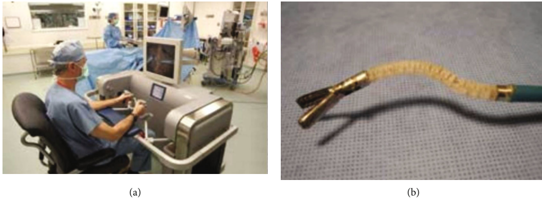
FIGURE 3: Master console and one of the mechanical actuation arms of the ViaCath system [7]: (a) master console and (b) mechanical actuation arm.
