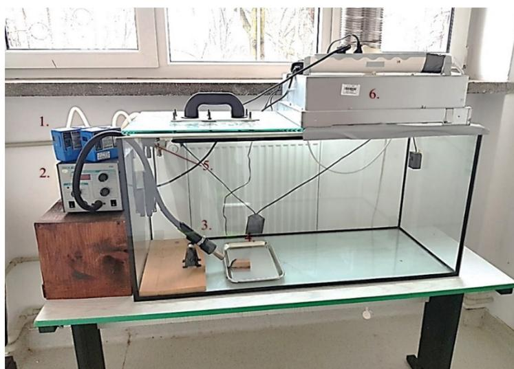
**Figure 1.** Measuring stand: 1—GilAir-3 personal aspirators; 2—device regulating heat release; 3—source of radiation; 4—tray with tested combustible material; 5—heads for collecting respirable and total suspended particle (TSP) fractions; 6—exhaust smoke.
