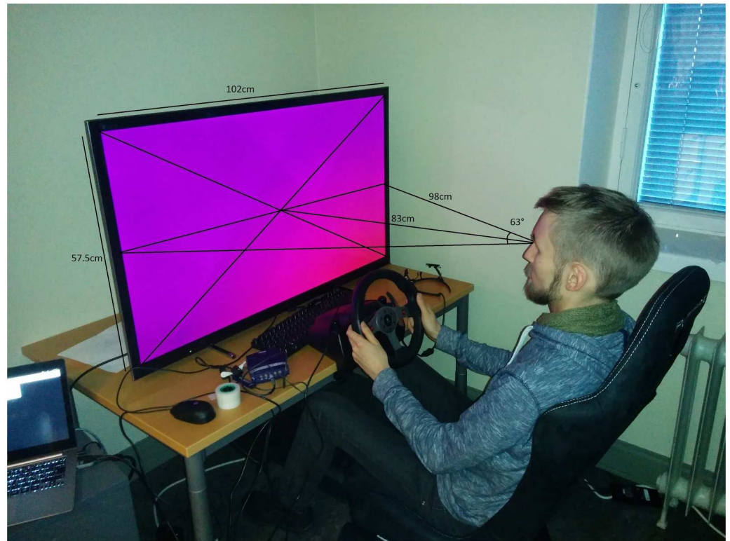
Fig 1. The physical setup of the driving simulator.
