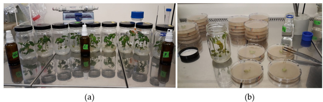
Figure 6. Inoculation of Phytophthora infestans on susceptible potato cultivar Dobrin in vitro. (a) Four to five week old in vitro plantlets of Dobrin were used to maintain virulence of P. infestans isolates before experiments. Zoospore suspension was inoculated using 50 mL glass spray bottles. (b) Five to six days post inoculation mycelium-covered leaflets were transferred to Rye-A+ medium.
