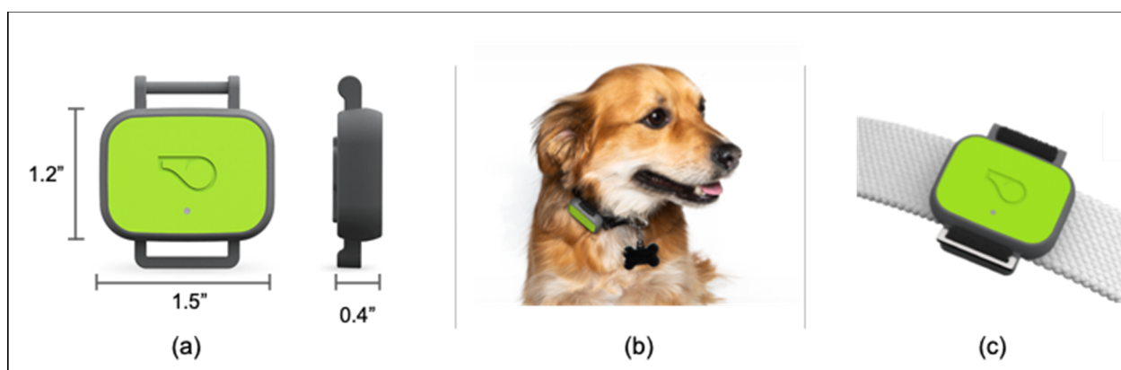
Figure 1. Activity monitors used in this study. Most data in this study were acquired from Whistle FIT ® activity monitors. Device dimensions are shown in (a), and a device in use is shown in (b). The device often rotates to different positions around each dog's collar. The device can attach to most dog collars up to 1" (25 mm). Attachment detail is shown in (c). The two other devices used this study (the Whistle 3 ® and the Whistle GO ® ) are larger and heavier.
