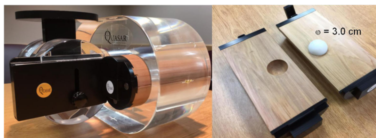
Fig. 1 Quasar respiratory motion phantom with cedar lung insert and offset polystyrene sphere 3.0 cm in diameter
