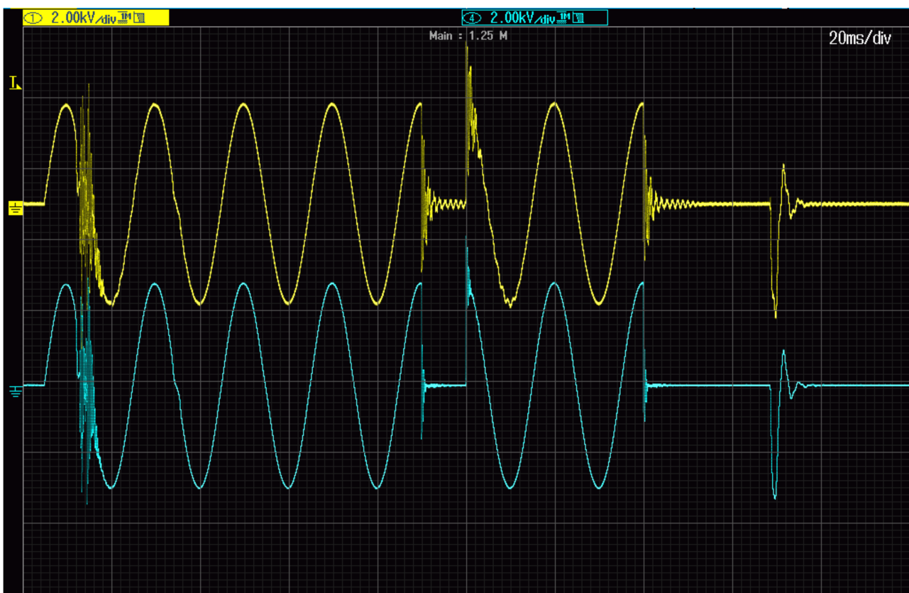
Figure 6. Voltage waveforms of voltages on primary (blue line) and secondary (yellow line) windings of the 2 kV step-up transformer.
