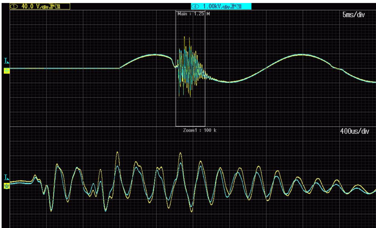
Figure 9. Voltage waveforms of voltages on primary (blue line) and secondary (yellow line) windings of the 15 kV voltage transformer.
