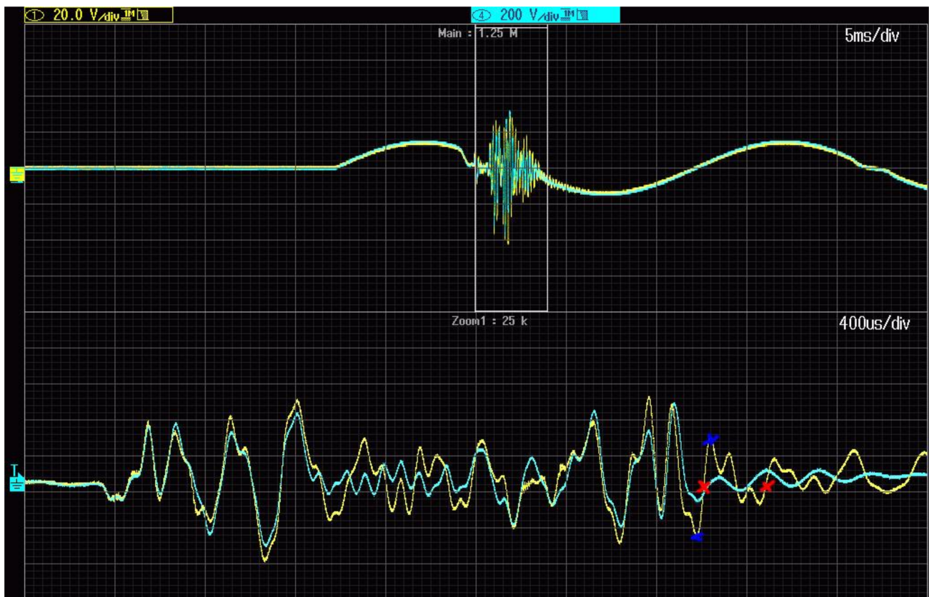
Figure 7. Voltage waveforms of voltages on primary (blue line) and secondary (yellow line) windings of the 20 kV inductive VT (model 1).
