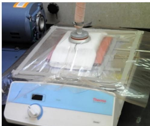
**Figure 8.** Photograph of the vacuum bagging mold assembly.
