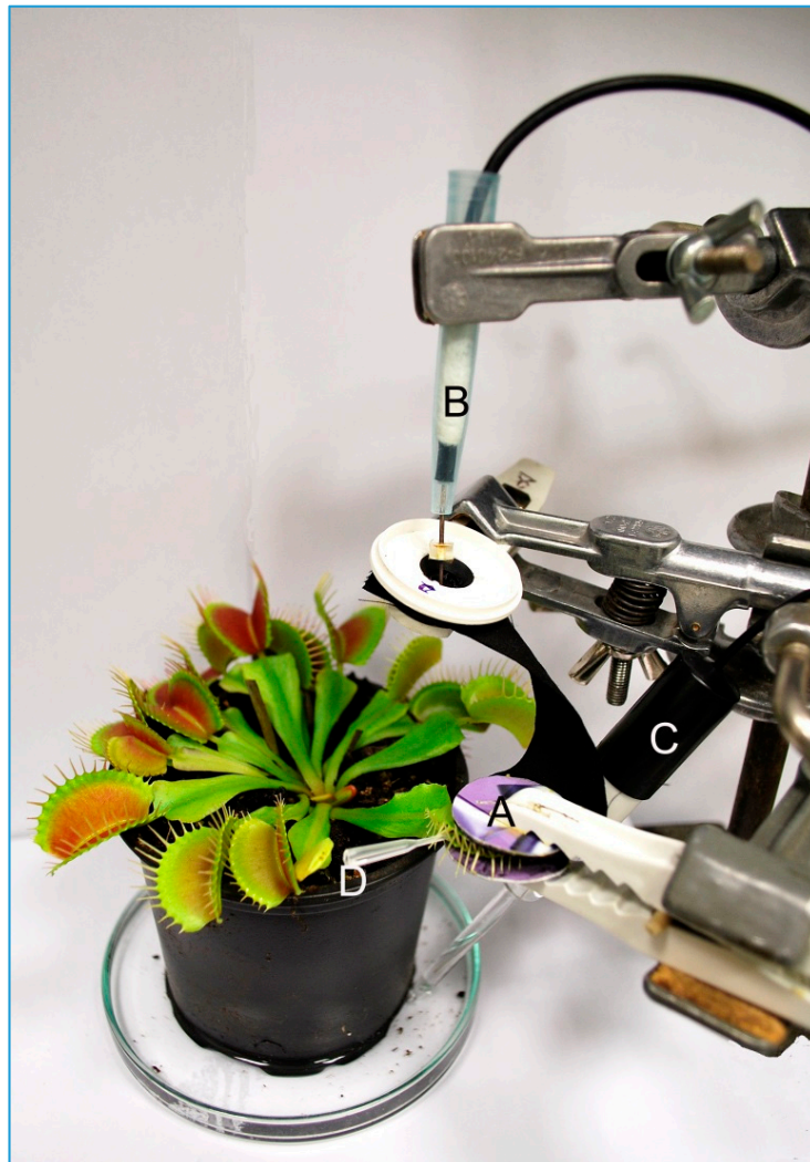
Figure 7. The layout of the electrodes used for recording of action potentials: clip electrode with cotton fabric coated with conducting polymer (A); non-polarizable Ag/AgCl surface electrode connected to the protruding strip of cotton fabrics coated with conducting polymer (B); and reference electrode (C); A plastic stick was used for stimulation of trigger hairs inside closed trap of Venus flytrap (D).
