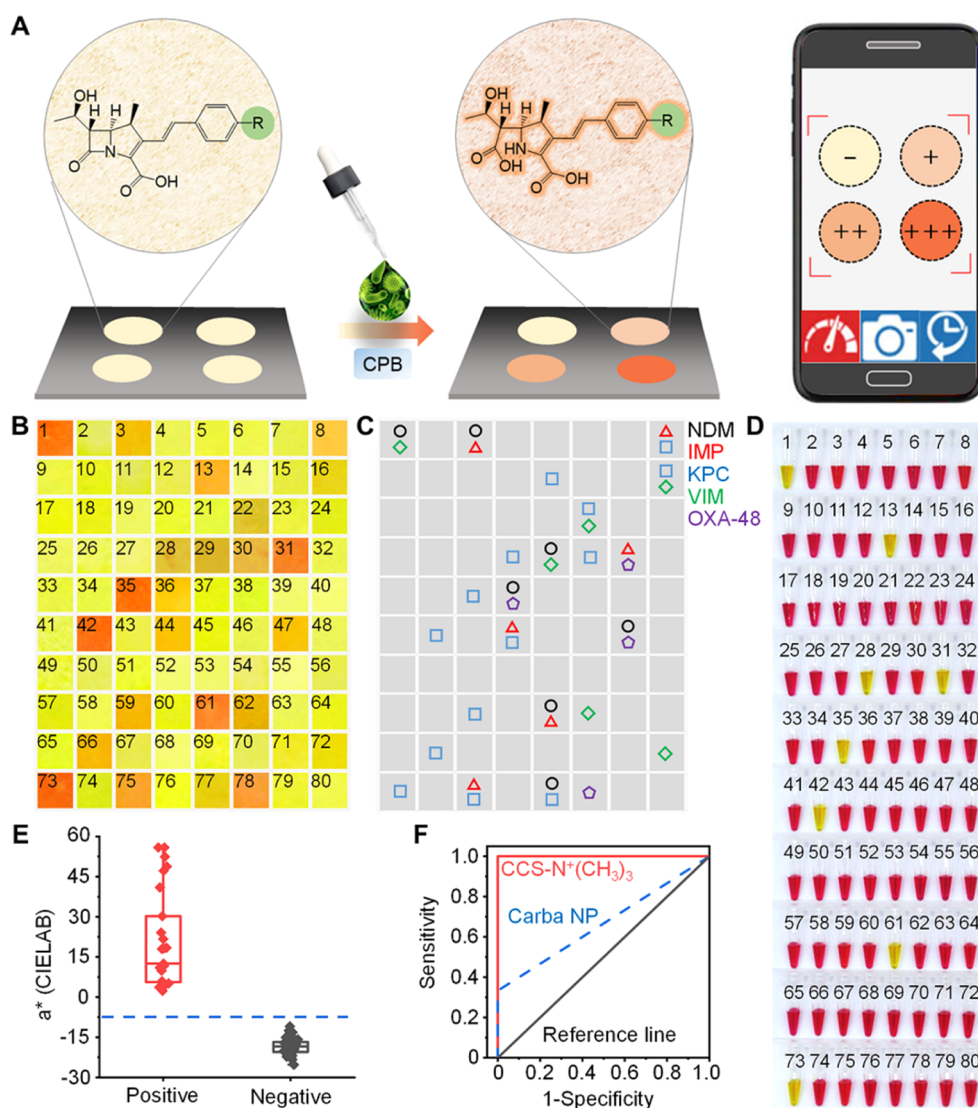
Figure 4. Detection of CPB in the clinical sputum samples collected from lung-infected patients. (A) Schematic of visual detection of CPB on a paper chip, where the color changes can be quantitatively identified by a smartphone installed with a color recognizer software. The a^* values reflecting colors from green to red were recorded in the CIELAB (Lab) color model. (B) 80 culture-free sputum samples detected by the \text{CCS-N}^+(\text{CH}_3)_3 -loading paper chips. (C) Carbapenem-resistant genes in the same culture-free 80 samples analyzed by RT-PCR. Each square corresponds to the paper block in (B). (D) Carba NP test (solution B) toward the same 80 cultured samples at 2 h (the results of solution A are provided in Figure S58). (E) Statistics of the a^* values for the naked eye results in (B). (F) ROC curves of the \text{CCS-N}^+(\text{CH}_3)_3 -based POC method and the Carba NP test.
