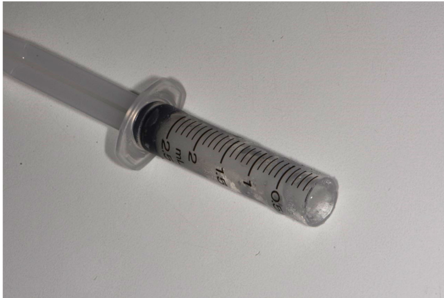
Fig. 4 Ice-filled syringe after cutting off the tip
