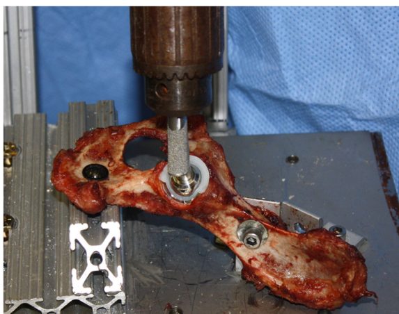
Figure 4 Specimen testing set up of the hemipelvis with implanted acetabular cup loaded to failure at a standing angle using a prosthetic femoral head and stem.
