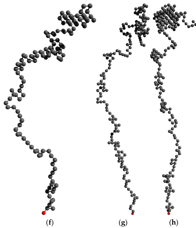
Figure 7. Typical chain conformations in the system with DP_n = 160 : m = 90 (a), m = 130 (b), m = 180 (c), and m = 230 (d). Enlarged typical single-chain conformations are also presented: (e) for (a), (f) for (b), (g) for (c), and (h) for (d).
