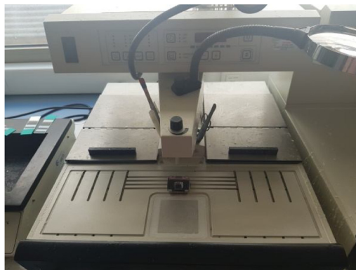
Fig. 2. Paraffin dispenser and embedding mold.
