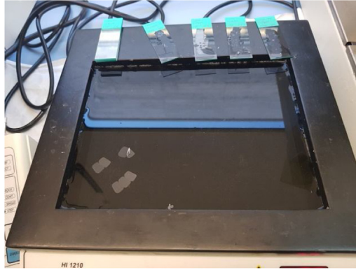
Fig. 3. Water bath set at 35 °C to stretch the paraffin sections.
