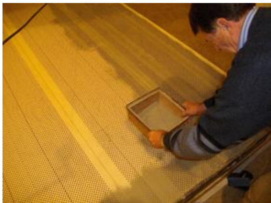
Figure 3. (a) Polluting of the sample with a sieve, (b) the sample after being sprinkled with cement dust in the amount of 5.0 \text{ kg}/12 \text{ m}^2 .
