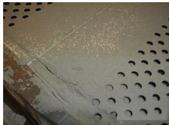
Figure 3. (a) Polluting of the sample with a sieve, (b) the sample after being sprinkled with cement dust in the amount of 5.0 \text{ kg}/12 \text{ m}^2 .
