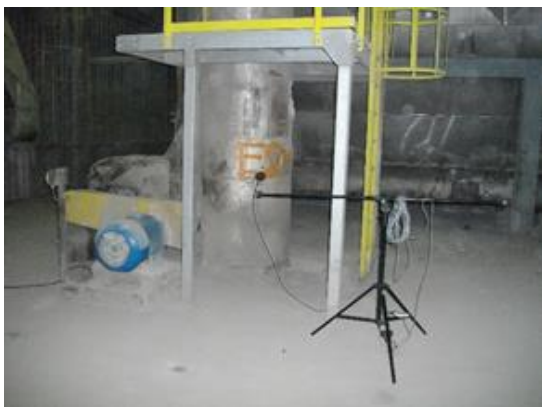
Figure 10. Immission measurement of sound pressure level from the fan in a cement plant production hall. (a) View of sound analyzer and the fan in the background. (b) Apart from the sound analyzer, the photo shows cement dust floating in the air indicating significant dustiness.
