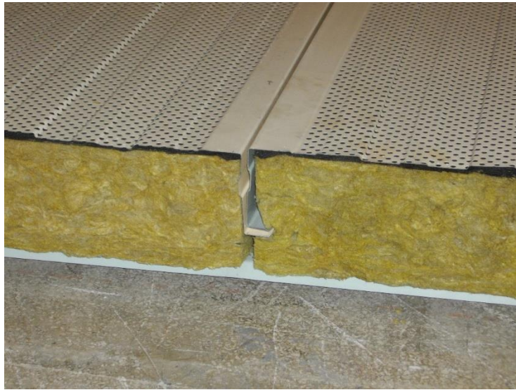
Figure 2. Fragment of the light curtain wall being the sample subjected to acoustic tests. Details of the test set-up on the floor of the reverberation room.
