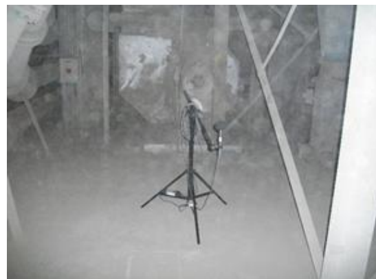
Figure 10. Immission measurement of sound pressure level from the fan in a cement plant production hall. (a) View of sound analyzer and the fan in the background. (b) Apart from the sound analyzer, the photo shows cement dust floating in the air indicating significant dustiness.
