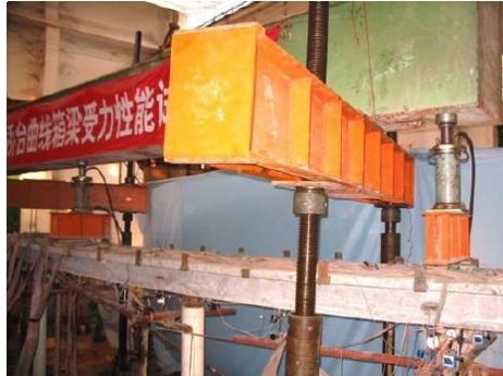
Figure 4. Experimental bridge model and loading apparatus.
