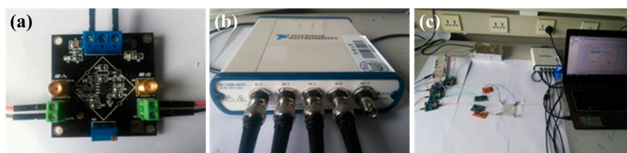
Figure 3. Measurement system of the touch panel. (a) OPA129 amplifying system; (b) NI-4431 four-channel data acquisition board; (c) The overall measurement system.
