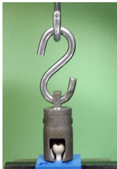
Figure 3. Trigger bell for the measurement of retention force, lined with a molded Teflon inlay.
