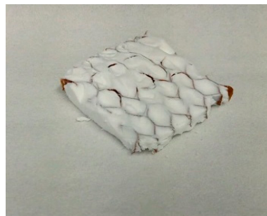
Figure 9. Low-flexible silica aerogel (SA2) with aramid honeycombs C1-6.4-24.
