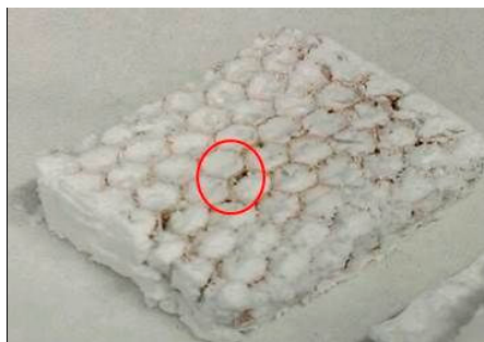
Figure 6. Super-flexible silica aerogel (SA1) with aramid honeycombs A10-92-5.2.
