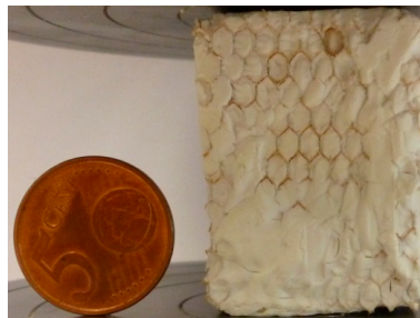
Figure 8. Low-flexible silica aerogel (SA2) with aramid honeycombs C1-3.2-29.
