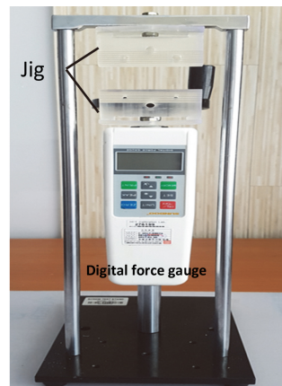
Fig. 4. It is a force measuring device by SH-500 (Digital force gauge, Sundoo, China). Force is measured from 1 to 50 N.
