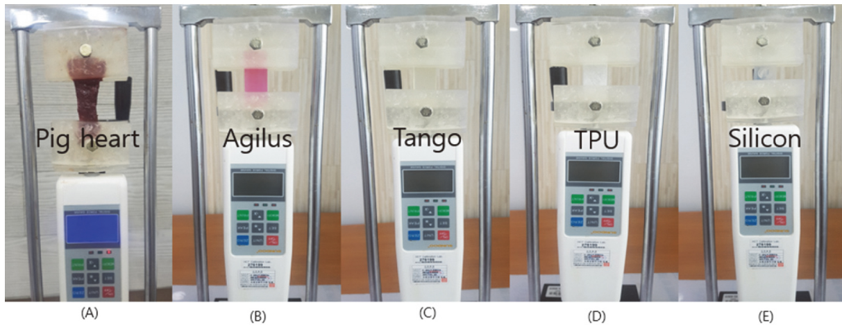
Fig. 5. Measure the change in length using a force of 5N (A) Pig heart elasticity experiment (B) Agilus elasticity experiment (C) Tango elasticity experiment (D) TPU elasticity experiment (E) Silicone elasticity experiment.
