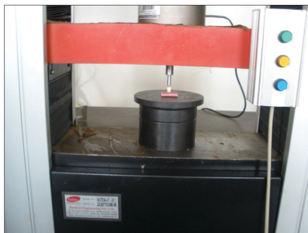
Figure 1: Specimen in the universal testing machine
