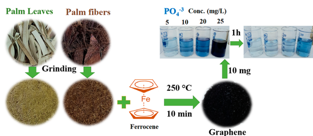
Figure 1. Schematic diagram and photos of the plant biomass and the synthesized ferrocene-functionalized rGO using the pyrolysis method and its application in the removal of phosphate from wastewater.
