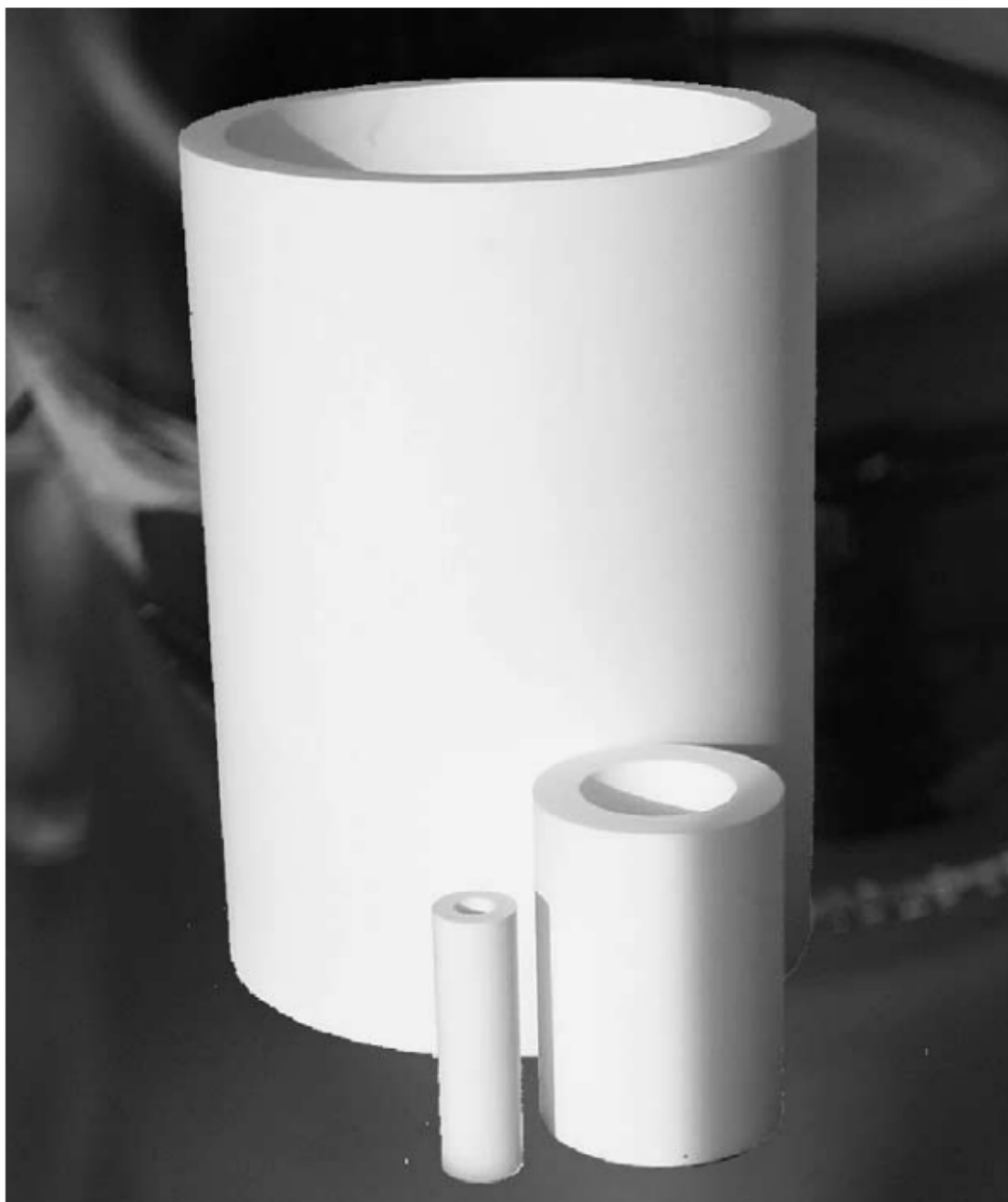
Figure 7. Radial flow CIM monolithic columns of different volumes (80, 800, and 8000 mL prototype), illustrating scalable designs for industrial applications. Reprinted with permission from Ref. [17]. Copyright 2005 Elsevier.
