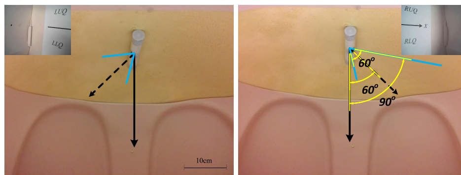
Figure 16. Tilt motion of the camera. A resultant tilt observation range angle of \pm 90^\circ was achieved.
