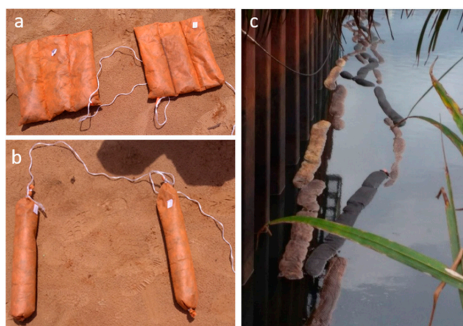
Figure 4. (a) Grafysorber ® pillows and (b) Grafysorber ® booms for American Petroleum Institute (API) oil-water separator test; (c) chains of Grafysorber ® and polypropylene (PP) booms in the channel.
