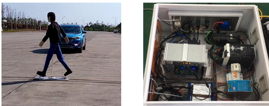
(a) Test scenario with a SUV and the dummy traction system (b) Base station of the cooperative control system
