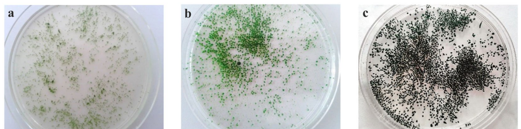
Figure 4. The time development of the granular activated algae system. Activated algae system during granulation process: (a) batch 59, (b) batch 122, and (c) obtained activated algae granules after 197 batches.
